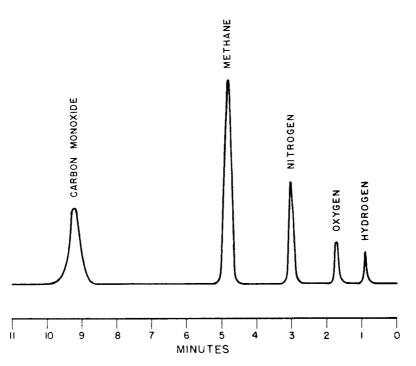
Column: 2-m by 6-mm inside diameter Type 13× molecular sieves, 14 to 30 mesh Temperature: 35°C
